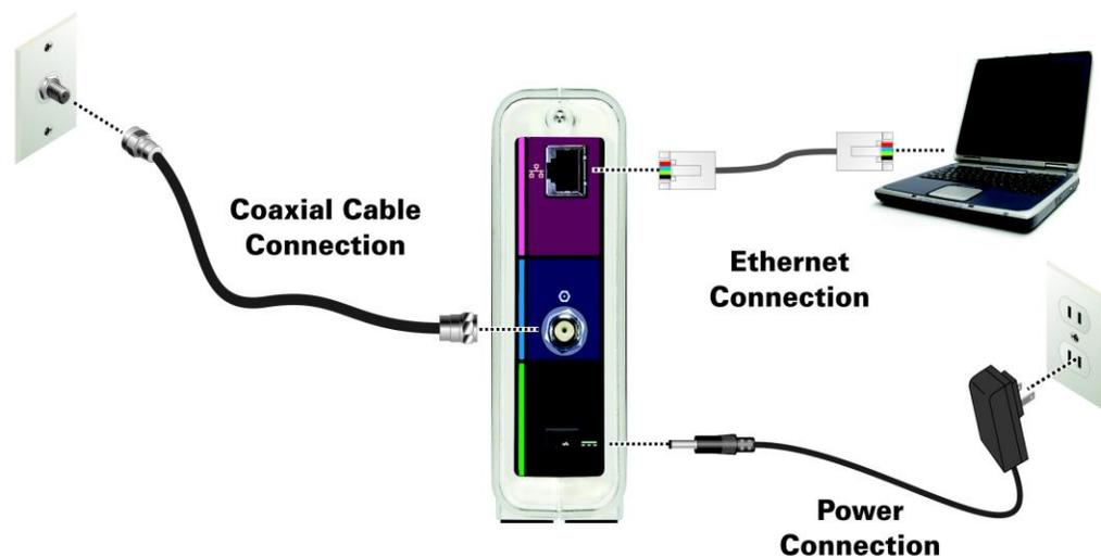
**Figure 3: SB6141 Connection Diagram**
